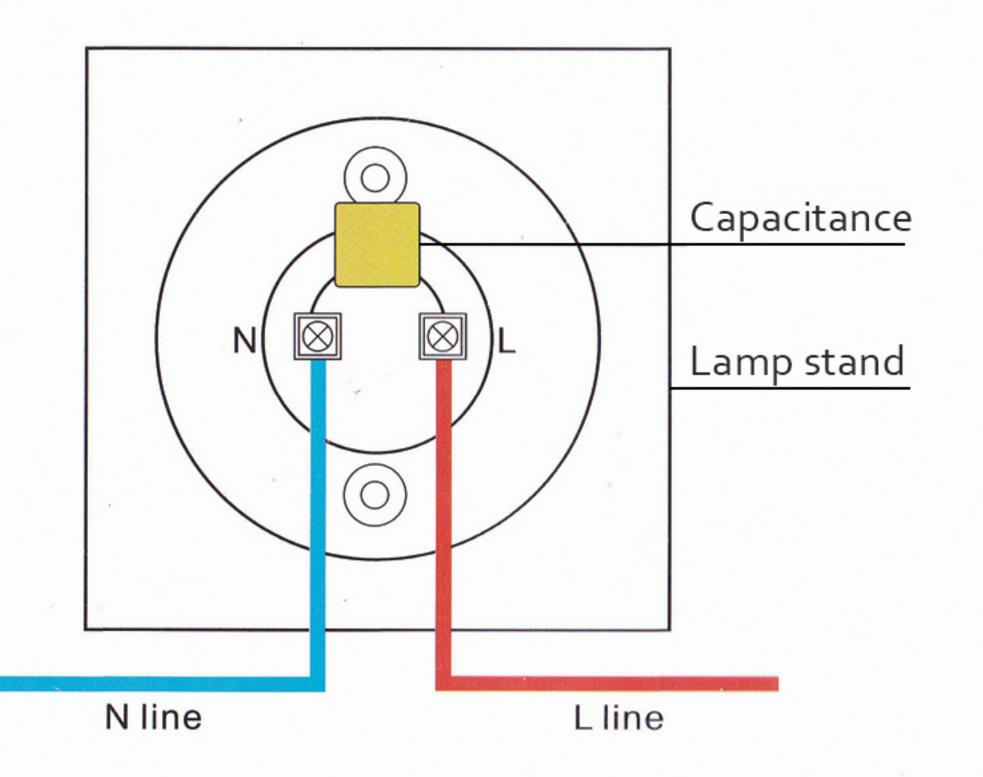
When the lamp Micro-light or start flashing, Please connect the capacitance between L line and N line. as shown in the drawing.
