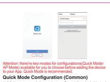
Make sure quick mode configuration is initiated the indicator light blinks blue rapidly (twice per second). If it blinks blue slowly (once every 3 seconds), press and hold the power button on vour Smart Switch for 20 seconds until the indicator light blinks rapidly.
